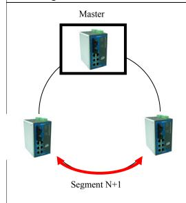
If the number of Ethernet switches in the Turbo Ring is 2N+1 (an odd number), the backup segment is the (N+1)st segment counting counterclockwise.
